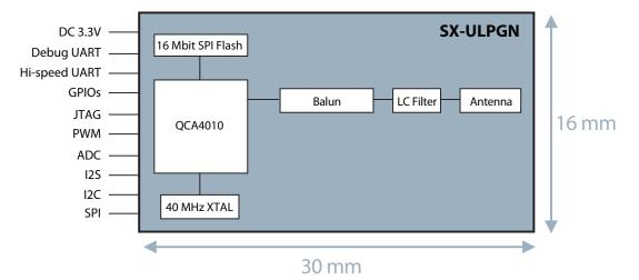
SX-ULPGN is based on the QCA4010 Reference Hardware & Software. The Software and documentation is available on the Qualcomm Developer Network:
